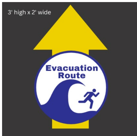
Figure 14 A preformed thermoplastic design of a tsunami evacuation route intended for use on asphalt roads in Puerto Rico (copyright PPG.com ).
