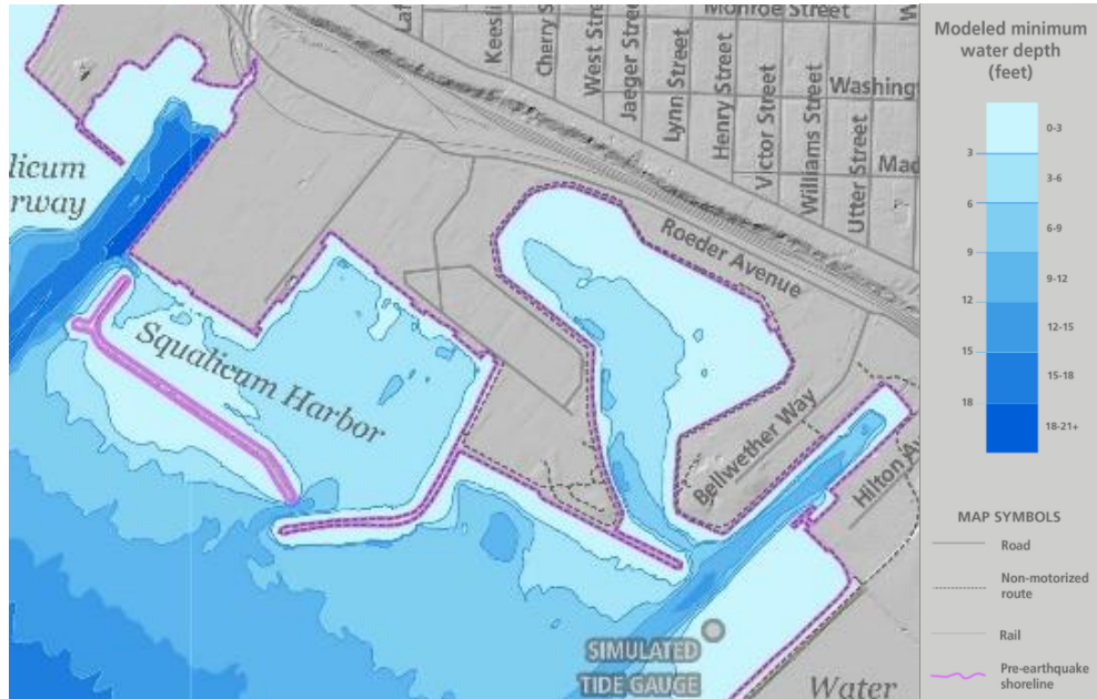
Figure 49: Close up of modeled minimum water level from distant tsunami at Squalicum Harbor, for full map see figure 23.
