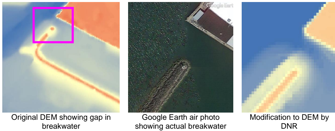
Figure C1. An example of some of a modification done to the Bellingham 1/9 arc-second DEM by WA DNR. Left: Closeup of the west entrance to the Outer Squalicum Harbor (pink square). The breakwater shows a gap that does not exist in the actual breakwater.
