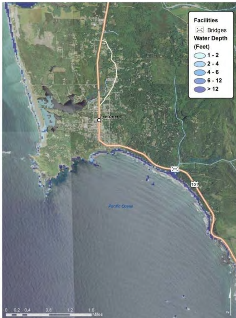
Figure B-44. Expected tsunami inundation and facility impacts for Port Orford, OR
