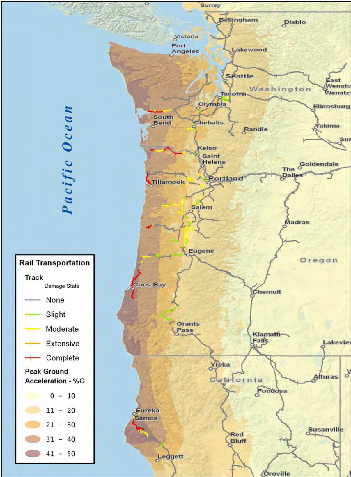
Figure 4-35. Damage to railroad track for the 50th-percentile (expected) case
