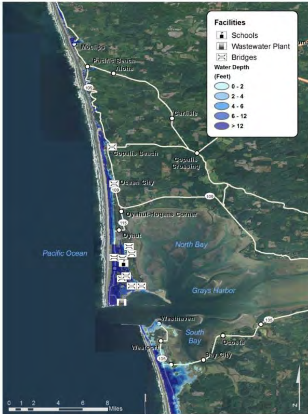
Figure B-66. Expected tsunami inundation and facility impacts for Moclips-Westport, WA
