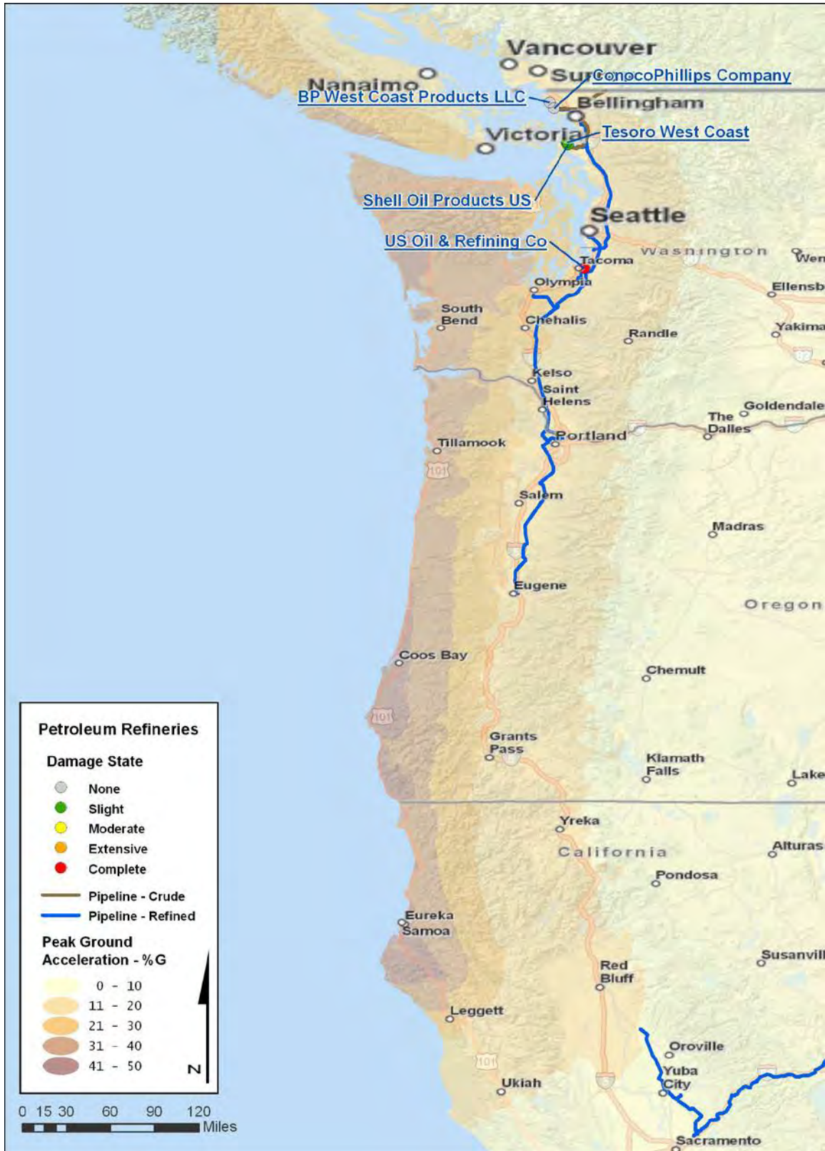
Figure 4-14. 50th-percentile (expected) case refinery damage levels
