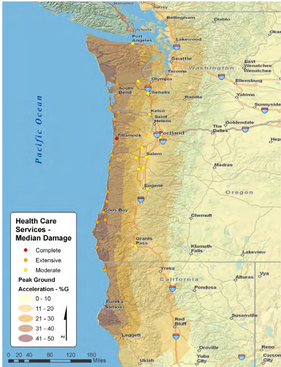
Figure 4-70. Hospitals located within the Cascadia region with expected damage states ranging from Moderate to Complete in the 50th-percentile damage case
