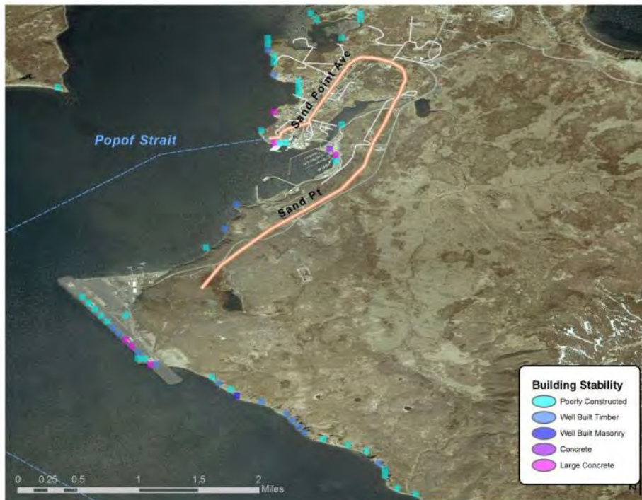
Figure B-11. Predicted building stability rating for Sand Point, AK
