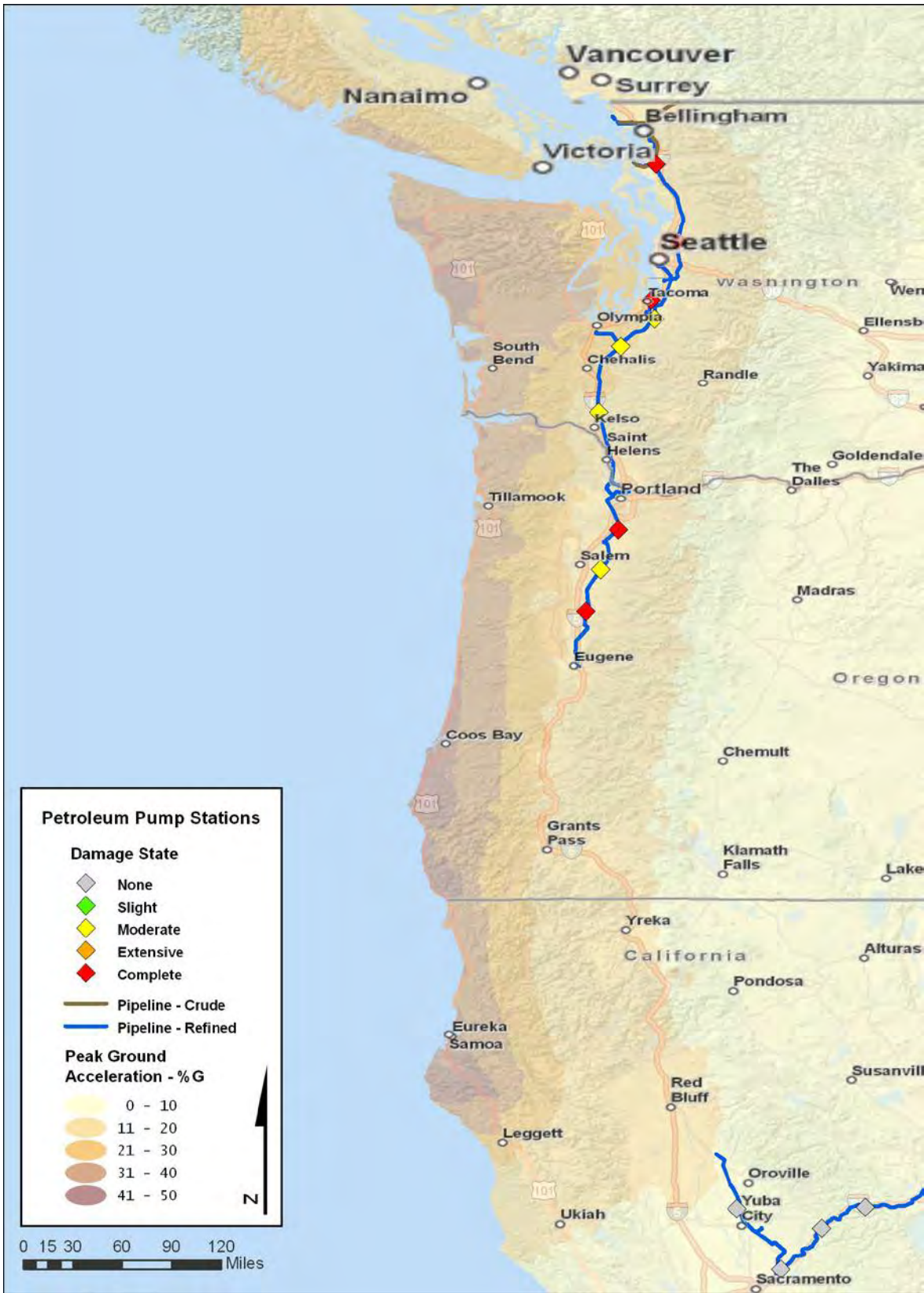
Figure 4-16. Petroleum pump stations damage level on day one
