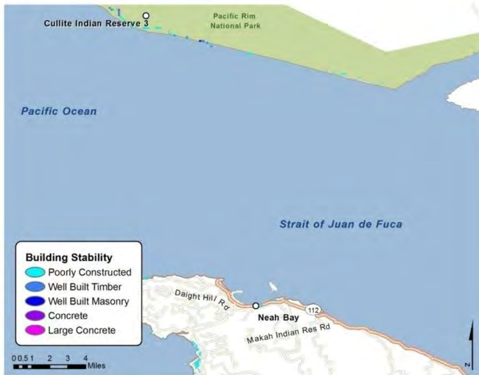
Figure B-68. Predicted building stability rating for Neah Bay, WA
