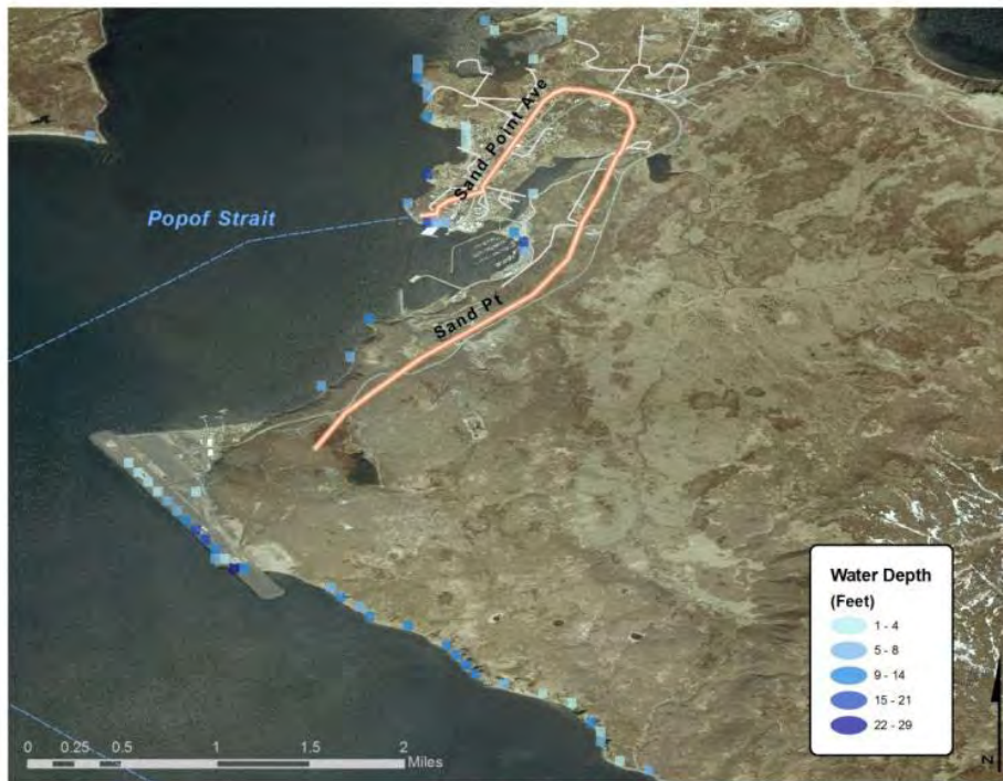
Figure B-10. Expected tsunami inundation depths for Sand Point, AK
