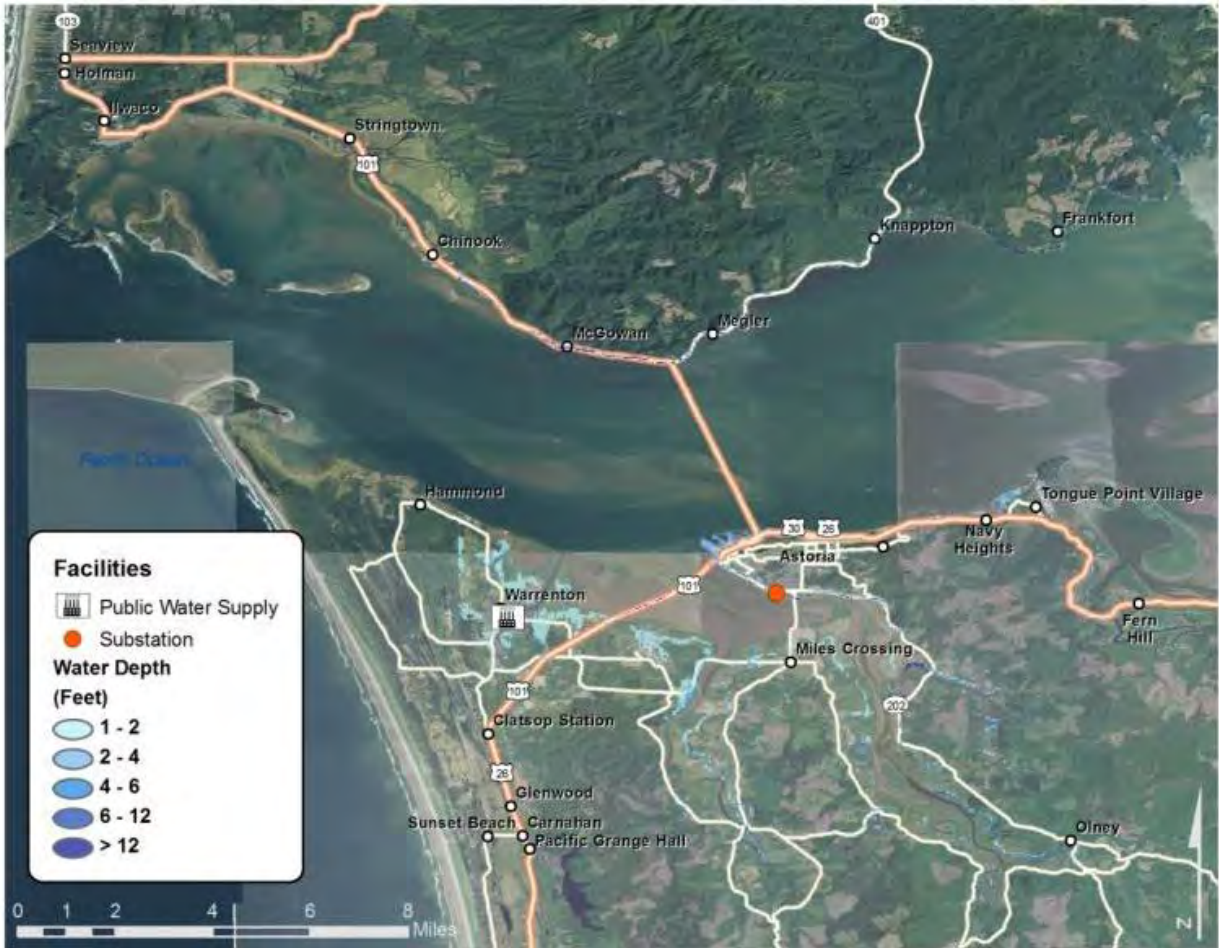
Figure B-38. Expected tsunami inundation and facility impacts for East Astoria, OR
