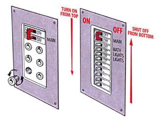
Always shut off all the individual circuits before shutting off the main circuit breaker.
