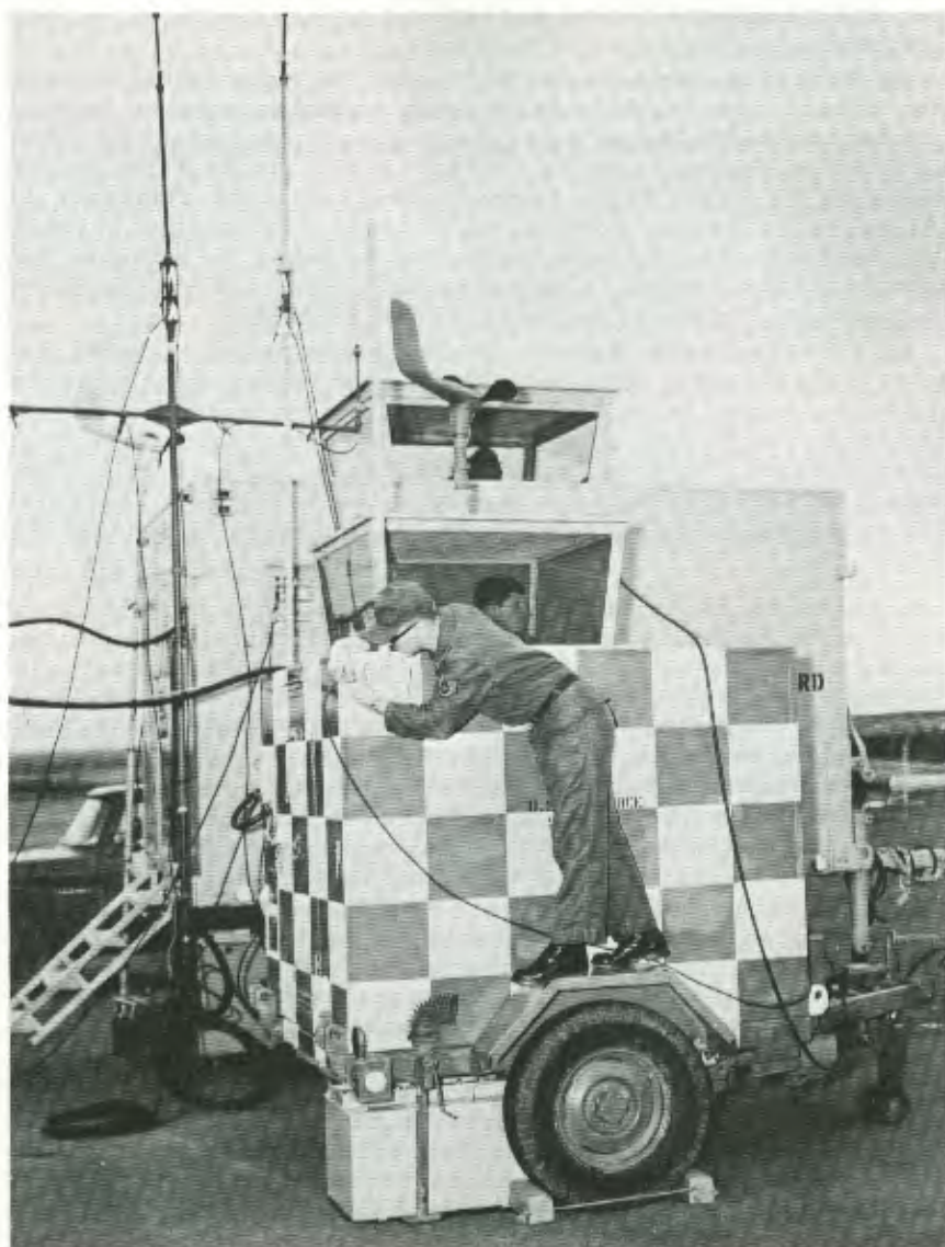
Air National Guard self-contained mobile control tower manned by 252nd Communications Group personnel for installation at unimproved forward bases.
