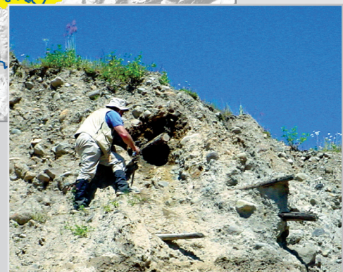
Geologists study the deposits of past lahars to assess potential future hazards. Here a U.S. Geological Survey geologist samples a log buried in a bouldery lahar deposit east of Enumclaw, Washington. This 5,600 year-old deposit, called the Osceola Mudflow, was formed when a massive landslide on the east side of Mount Rainier traveled north and west along the White River valley. (USGS photograph by A. Durant.)
