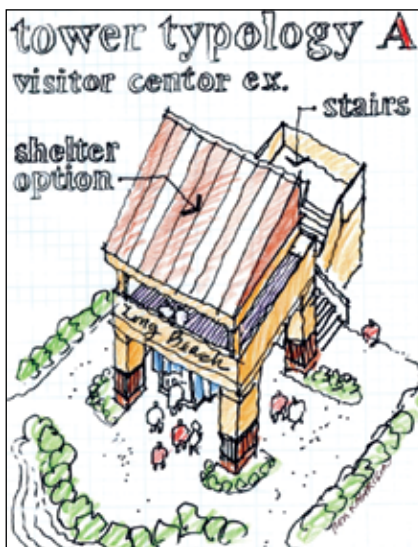
Figure 17: Basic tower structure A basic tower structure is a horizontal platform elevated above inundation levels by vertical supports. The at-grade level is open and can have additional rock or concrete barriers to break up wave-born debris. A “bare-bones” tower, essentially 40 feet square (200 person capacity) for example is a steel structure with a footprint of approximately 1,600 sf minimum.
