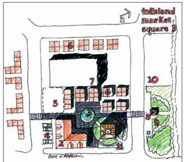
Figure 42: Tokeland Market Square Option Three Option 3 establishes a more formal community square with permanent and temporary facilities. Option 3 consists of (1) vertical evacuation facility viewing tower for bird habitat areas (views all directions with optional ground level tourism uses such as information center, display area; (2) community building with small meeting room, offices for Chamber of Commerce and other local organizations, and restroom facilities within building for security; (3) play and exhibit area with stage for musical events, with rock rubble wall on south and west faces; (4) staff/community building parking (seven spaces minimum); (5) relocated drain field; (6) temporary festival booths (seasonal); (7) existing port building; (8) ground level viewing shelter on waterfront; (9) small waterfront park area for bird watching; (10) parking and staging area for fisherman; (11) bird habitat area and water environment.
