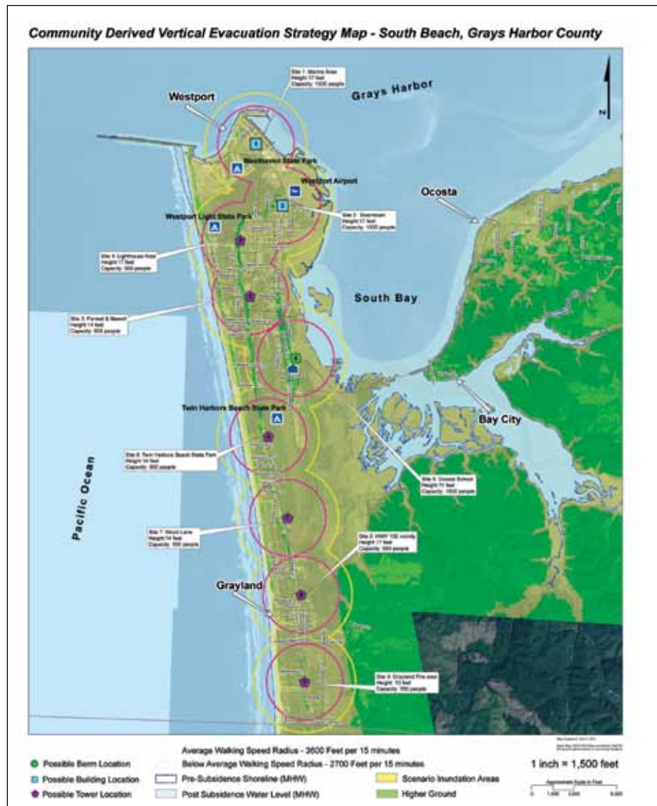
Figure 21: South Beach preferred community strategy. The map shows the vertical evacuation structures located throughout the peninsula, with their accompanying identification numbers.
