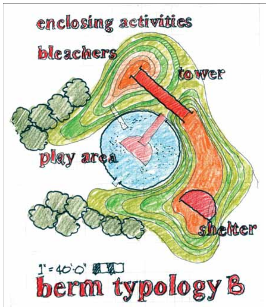
Figure 45: Berm typology B In this proposed example for Pacific County, a safe zone is embedded into a school berm. Play areas and events facilities can also be incorporated into and surrounding the berm structure.
