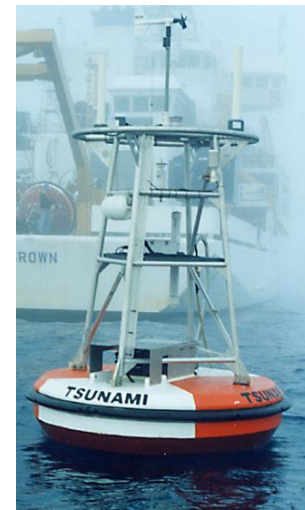
Figure 4 The first DART (Deep-ocean Assessment and Reporting of Tsunami) Detection Buoy
